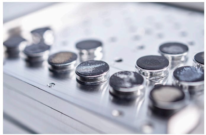
Sample holder with up to 30 12 mm pin stubs.
