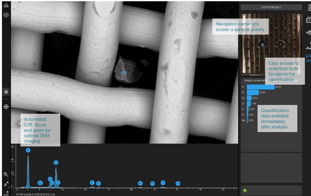
Figure 2. EDS capabilities embedded in the heart of the SEM UI. You can switch between analytics and imaging with a single click.
